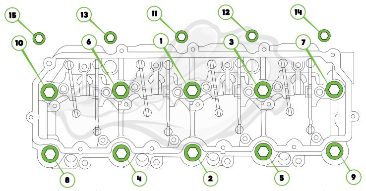
☐ The amount of Head Stud threads showing above the Head Stud Nut should all be about the same. If one appears to have more thread, the stud is most likely not all the way in the head.
