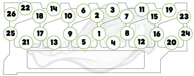
• The amount of Head Stud threads showing above the Head Stud Nut should all be about the same. If one appears to have more thread, the stud is most likely not all the way in the head.
